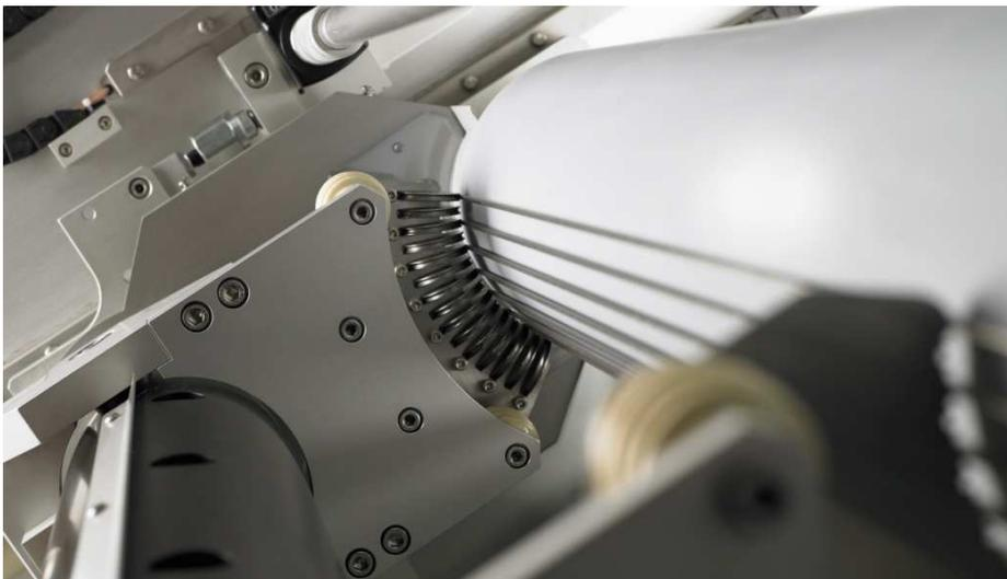
The open design and many small optimum technical solutions such as the quick release system for the BACK-UP electrodes facilitates fast and secure control of the system. With the unique calvatron® EMBEDDED design the IGBT generator is already directly integrated into the SX system. Therefore there is no need for additional space and cabinet.
