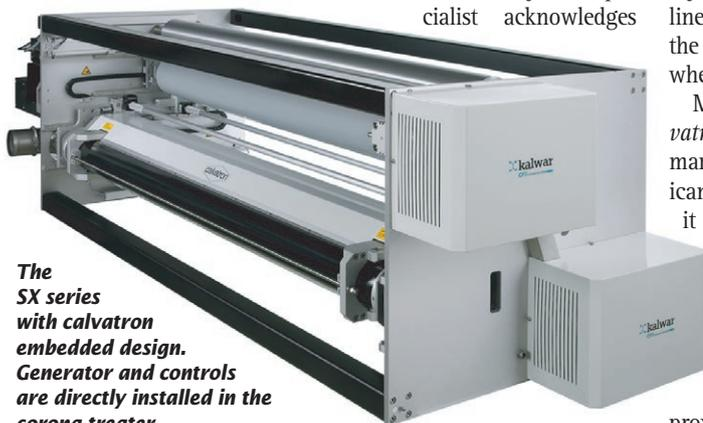
**The SX series with calvatron embedded design. Generator and controls are directly installed in the corona treater.**
