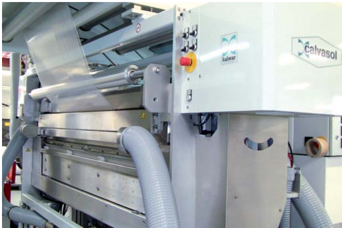
Abb. 2: calvasol® Serienanlage – Integration in einer Kaschieranlage Fig. 2: calvasol® series system – integrated in a laminating unit
